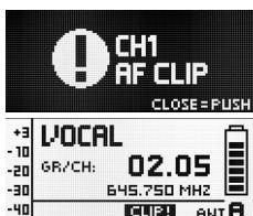
2. **AF CLIP:** Audio overload in transmitter A/D converter. The LED ring is lit red and a large warning message displayed for 5 secs. or as long as the fault condition lasts.
