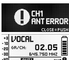
4. **ANT ERROR:** The same antenna has been active for more than one minute. The LED ring is lit red and a large warning message displayed for 5 secs. or as long as the fault condition lasts.
