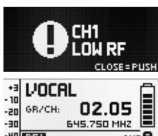
3. **RF LOW:** The field strength of the received RF signal is too low, the receiver's audio output is muted to prevent unwanted noise. The LED ring is lit red and a large warning message displayed for 5 secs. or as long as the fault condition lasts.
